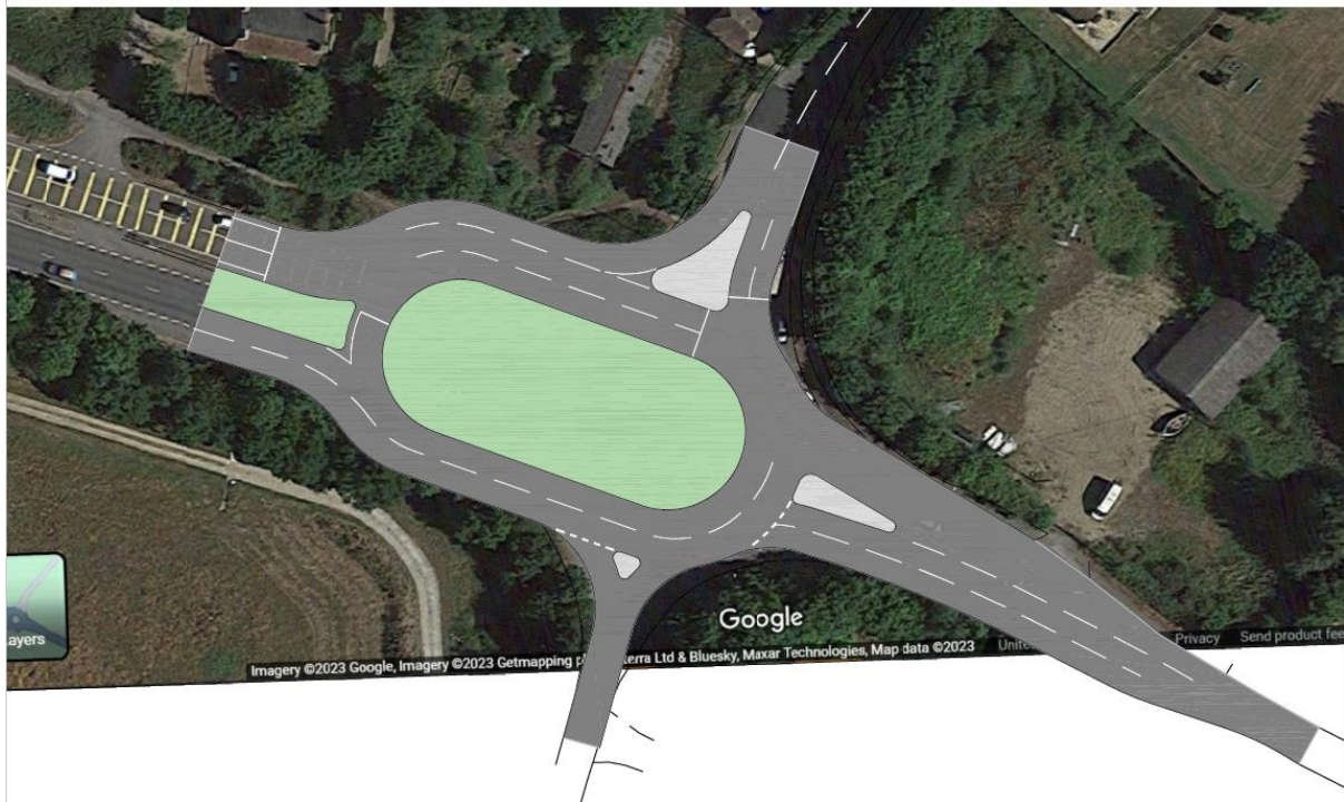
Figure 8-4 – Kippings Cross Partial Signalised Roundabout Junction
