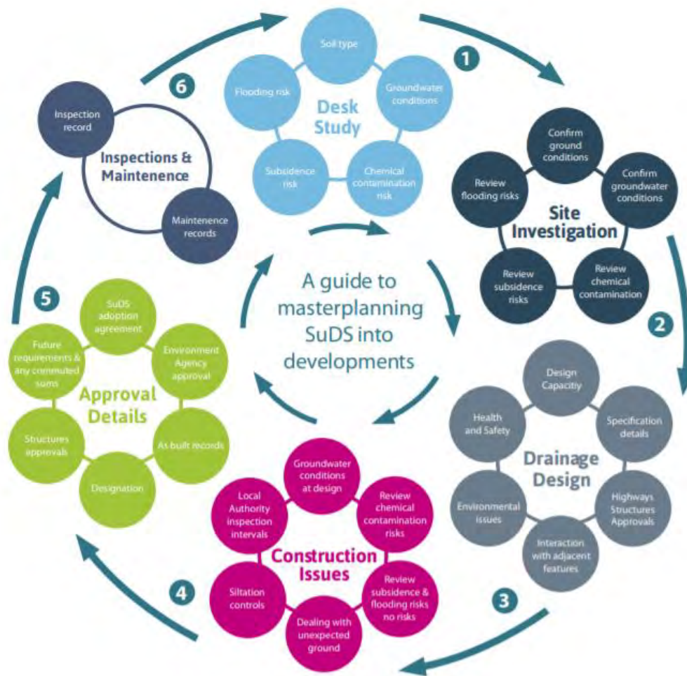
Figure 19: A guide to masterplanning SuDS into developments (source: Kent Design Guide – Making it Happen)
